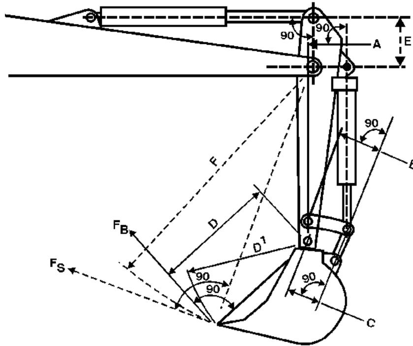
**$F_B$  = Radial tooth force due to bucket cylinder**
