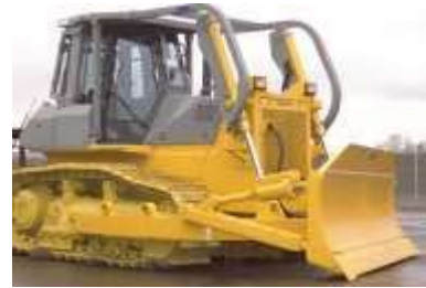
D65 Komatsu Extreme Service Angle Dozer c/w Dual Tilt Cylinders click on photo for larger view
